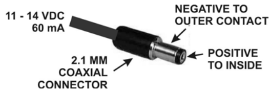
Figure 2. External Power Connector
